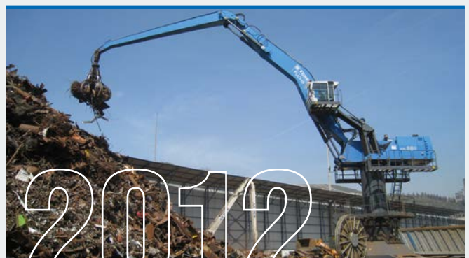
Largest electrically powered Fuchs material handler RHL880 D XL to date. Crawler undercarriage and pylon for maximum stability and overview during scrap handling.
