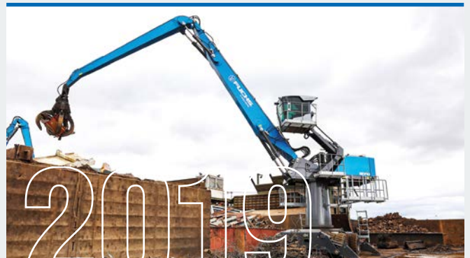
MHL870 F Pylon . Electric multi-talent in Mannheim harbour. From loading the ship to feeding the shear. All emission-free.
