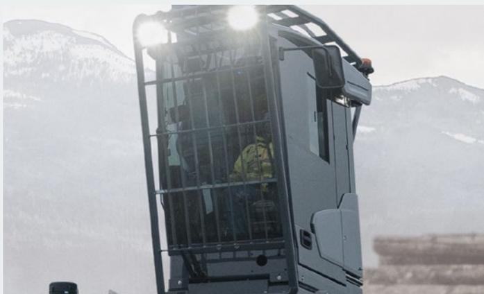
➔ Front and roof guard for timber application
