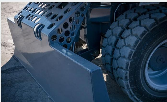
➔ Support blade, integrated cylinder protection
