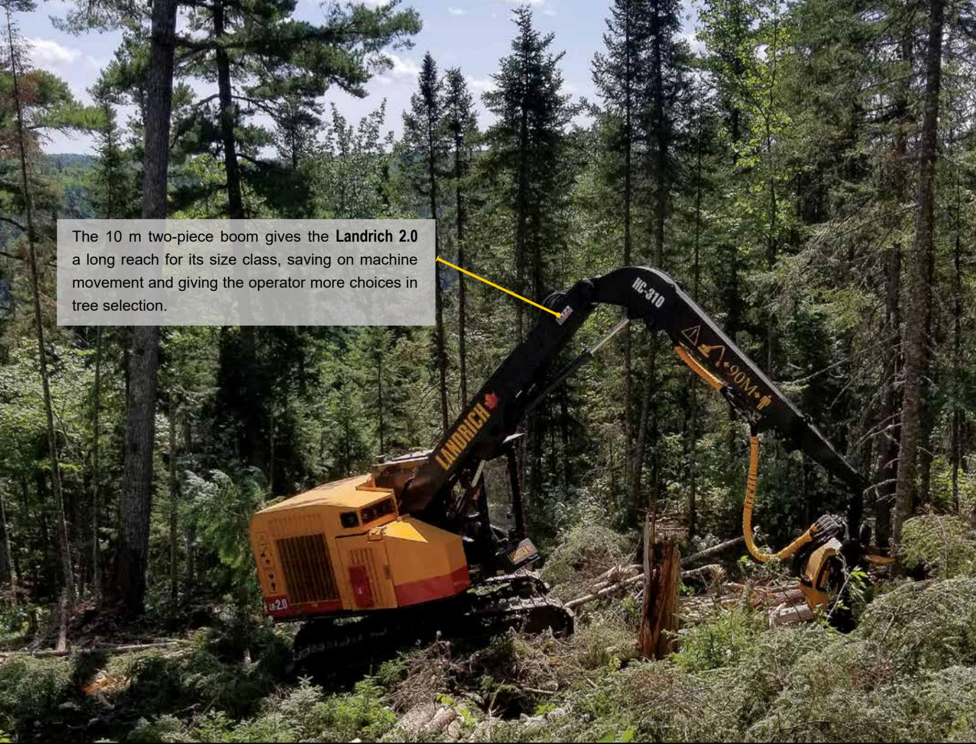
The 10 m two-piece boom gives the Landrich 2.0 a long reach for its size class, saving on machine movement and giving the operator more choices in tree selection.
